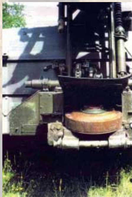
Mechanical minelayer mounted on the rear of a Soviet armored vehicle.
