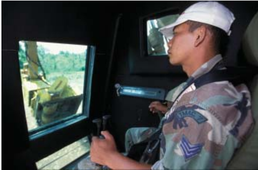
This mechanical assistance machine operator clears mines from behind armored glass and steel plate protection.
