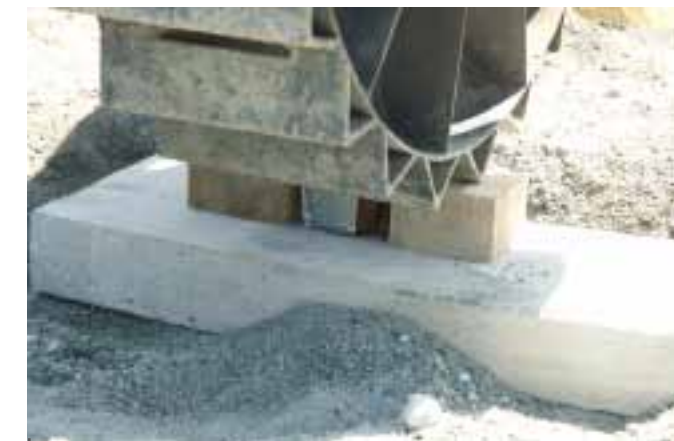
Figure 5. Placement of the charge underneath the wheel and thermalite block.
