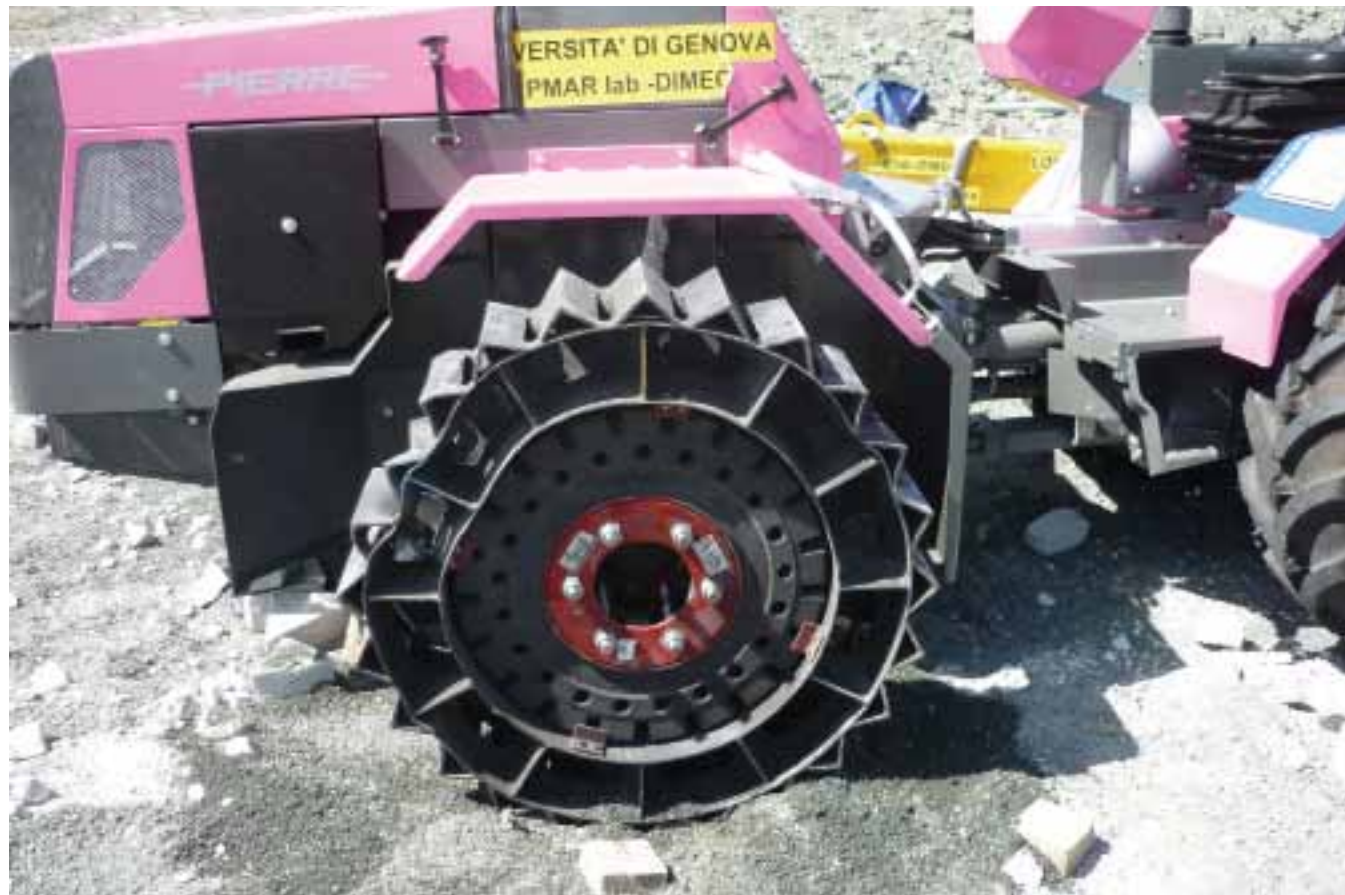
Figure 11. Genoa wheel after the fourth explosion. Only this last test was done on
